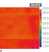
4 hours after switching on: T average surface module 28.1°C.
